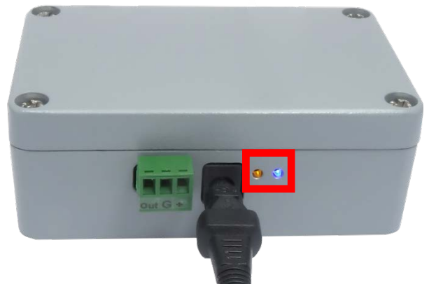
Image 12: Readers's LEDs working
