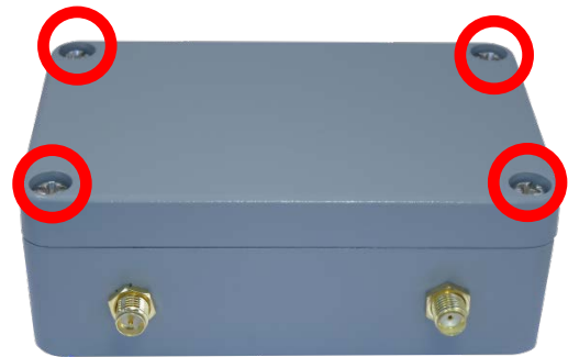
Image 8: 4 screws to be unscrewed
